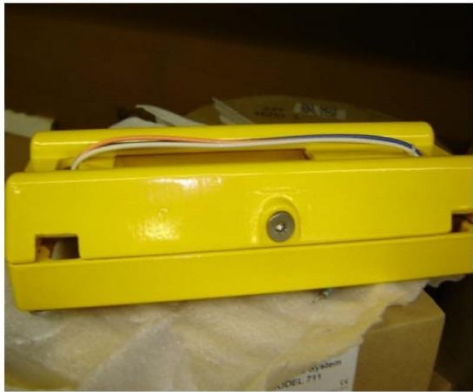
Picture 3 – clamshell mount bracket with flat head 3/16" hex socket closure bolt
